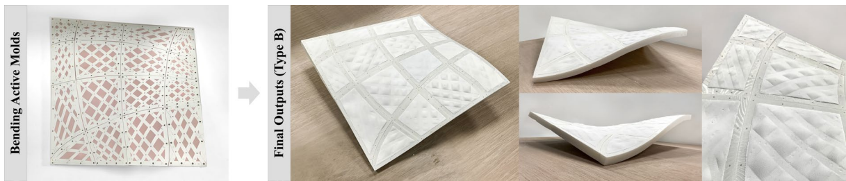
Figure 15: Fabrication results for Type B before and after mold removal
