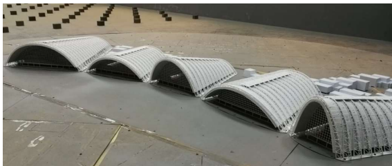
Figure 6: Wind tunnel vault models
