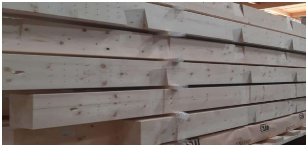
Figure 10: Unique arch segments with notches for purlins
