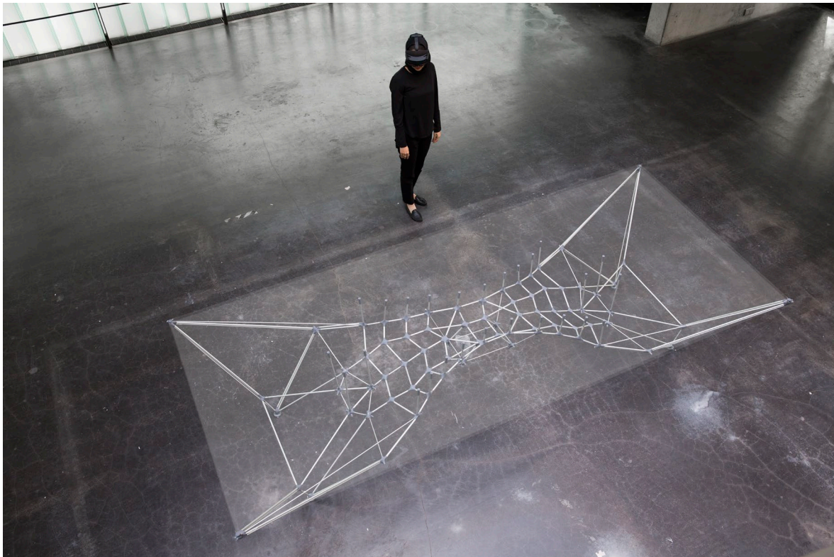
Figure 8: Final assembled table substructure with virtual tabletop.
