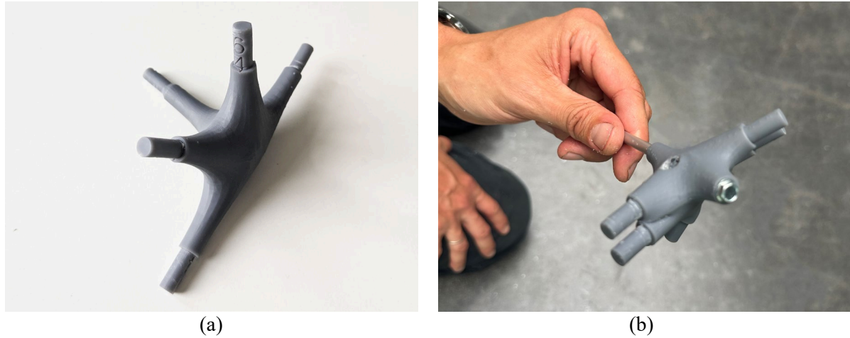
Figure 4: Additive manufacturing of the generated joints: (a) connections to the compression rod elements incorporate a plug-in mechanism; (b) connections to the tension rod elements utilize a combination of push-through and screw strategy.
