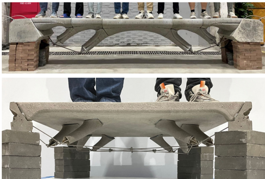
Figure 6: Beam and floor prototypes by Tongji University and RMIT University: top) “FloatArch”; bottom) “FloatSlab” [24].
