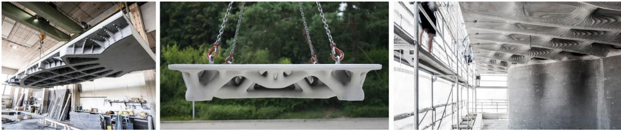
Figure 2: Optimised concrete floor slabs built by: left) Graz University of Technology [2]; middle) Digital Building Technologies, ETHZ [10]; right) Digital Building Technologies, ETHZ [11].
