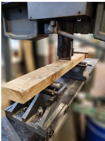
Figure 4: 3-points bending test – wooden board [5.7x14 cm 2 ]
