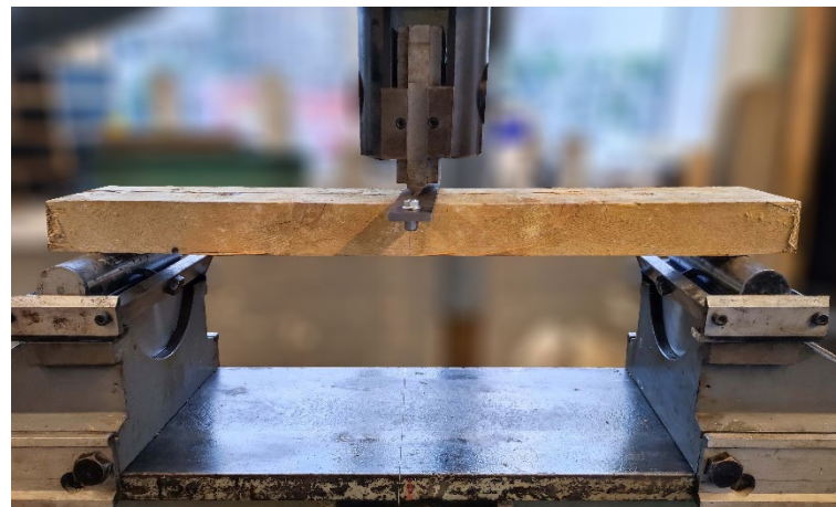
Figure 5: 3-points bending test – wooden board [5.7x14 cm 2 ]
