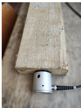
Figure 7: NDT with an ultrasonic pulse velocity device
