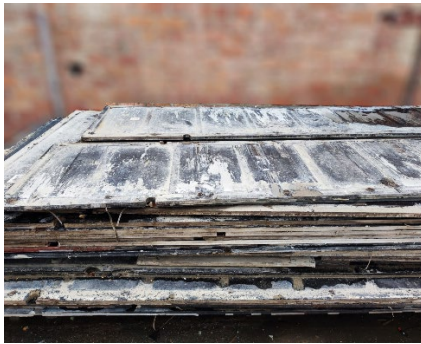
Figure 1: batch of used multiplex wood on construction site
