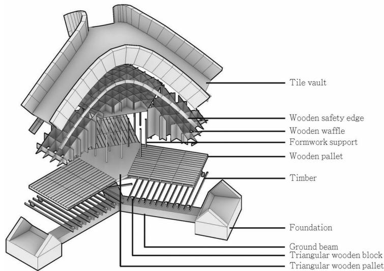
Figure 4: Overall vault construction review
