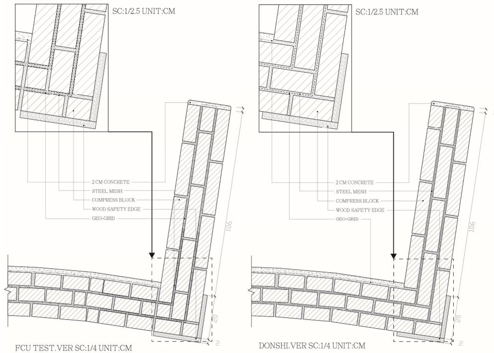
Figure 3: 1:1 Design detail, Feng Chia University prototype testing detail with plastic geogrid, and Dongshi Forestry Cultural Park potential construction detail with steel wire.
