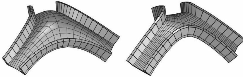
Figure 2: RhinoVault2 generated design (Left) and Kangaroo 2 Physics generated design (Right)
