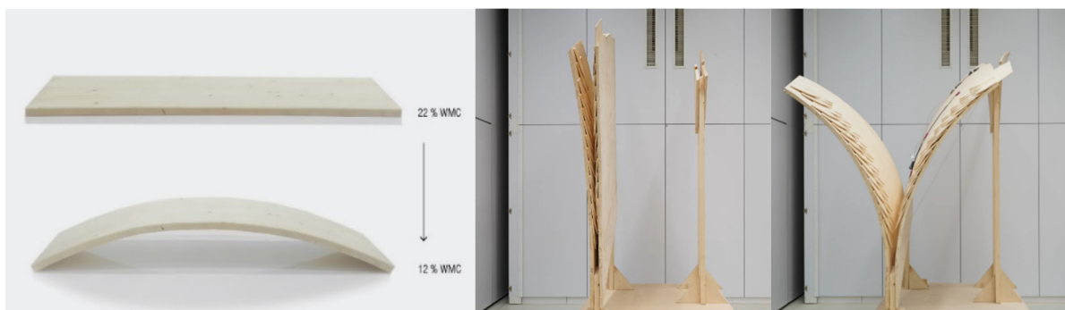
Figure 2: (a: left) Self-shaping of a single board Source [5]. (b: right) self-shaping of a test package developed for HygroShell.
