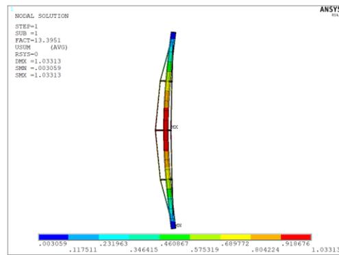
Figure 8: Overall buckling mode of cable column
