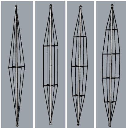
Figure 9: Cable column models with different number of struts
