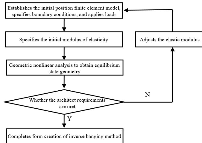
Figure 4: Numerical inverse hanging method flow chart
