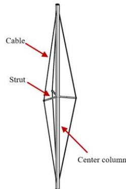
Figure 7: Structural drawing of cable column
