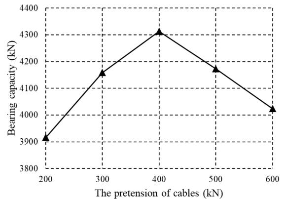
Figure 14: Effect of cable pretension on the bearing capacity
