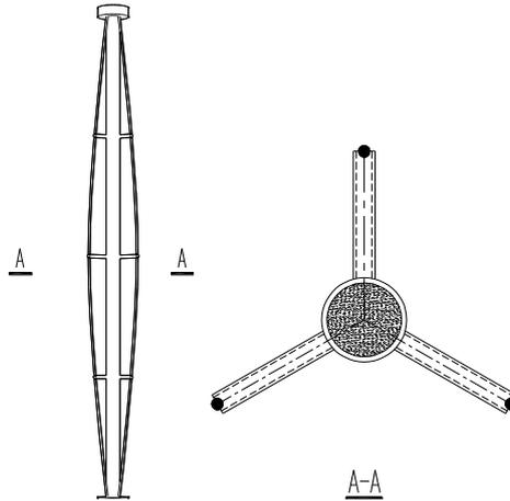
Figure 15: Drawing of pre-tensioned cable column of this project
