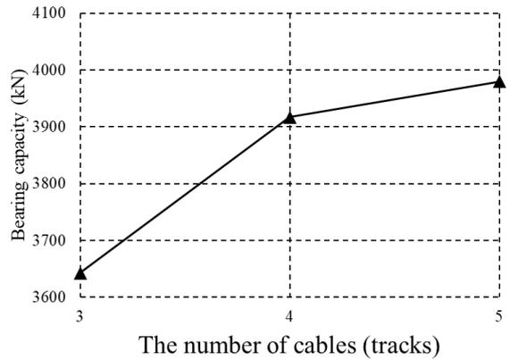
Figure 12: Effect of the number of cables on the bearing capacity
