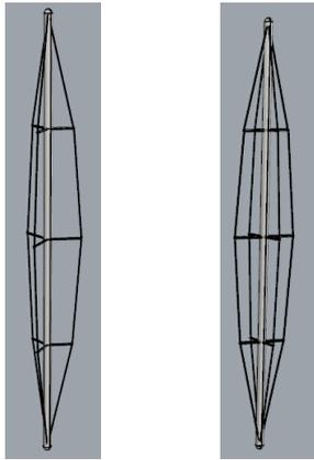
Figure 11: Cable column models with different number of cables
