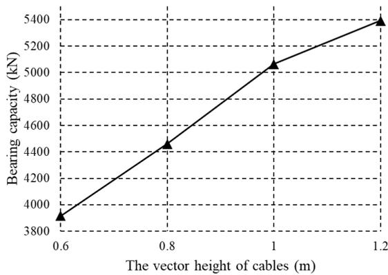
Figure 13: Effect of cable sagittal height on the bearing capacity
