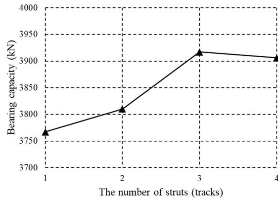
Figure 10: Effect of the number of struts on the bearing capacity
