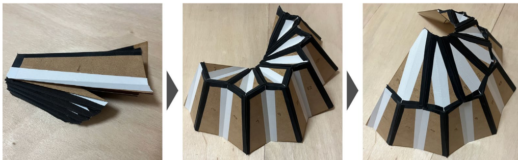
Figure 9: The deployment of the thick-panel model made of MDF.
