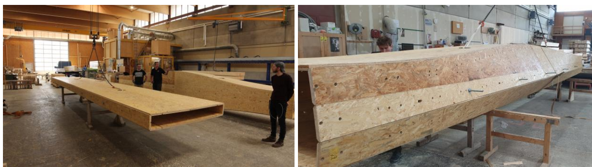
Figure 10: One beam in flat state, and on in folded state in the back ( left) and the beam during actuation (right)
