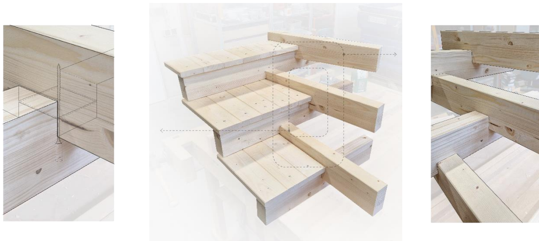
Figure 11: close-up Detail of the joint and the 1:1 Model of a bridge section of the Timber beams on a 3-Axis CNC
