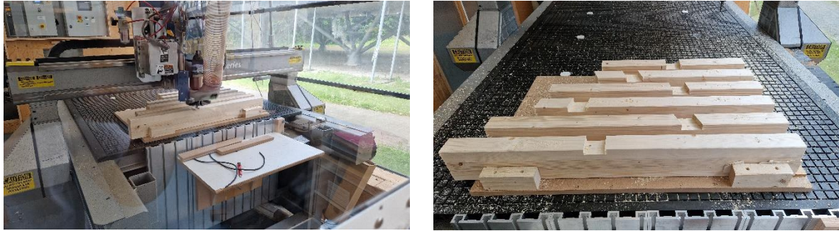
Figure 10: machining of the Timber beams on a 3-Axis CNC
