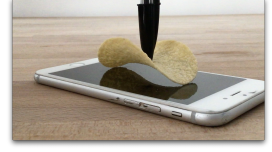
(d) Point load test of a model from a packet of Pringles® using a BIC® Biro or ballpoint pen.
