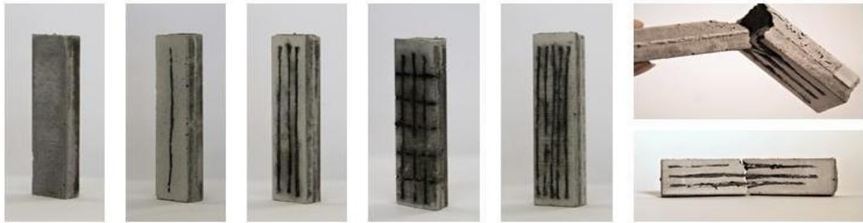
Figure 6: Left: Fabricated samples before structural test, Right: Fabricated samples after structural test
