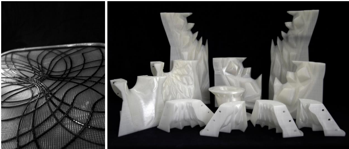
Figure 13: Regions of formwork incorporating CFRP reinforcement
