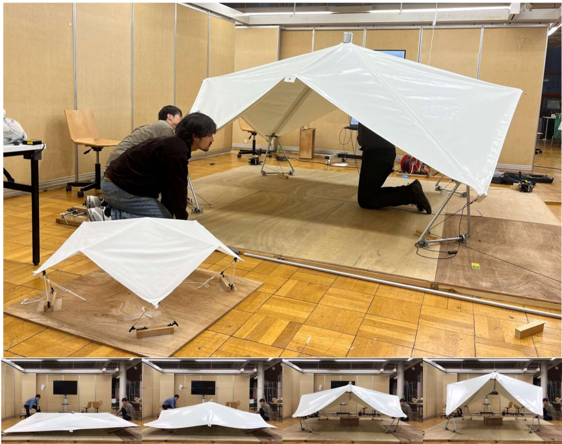
Figure 11: Mock-up made of shortened CFRP and adjusted so that the membrane is applied in the same shape as the scale model, and its deployment process.
