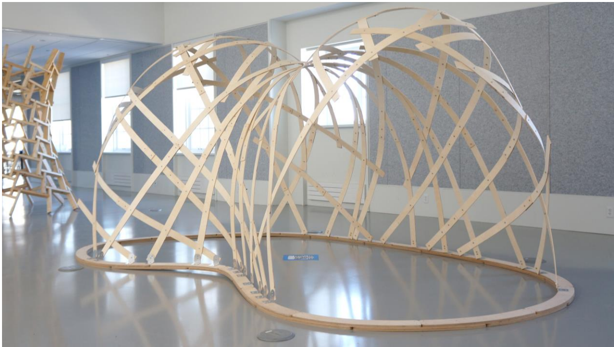
Figure 1: Ad-hoc geodesic gridshell prototype built in mixed reality.
