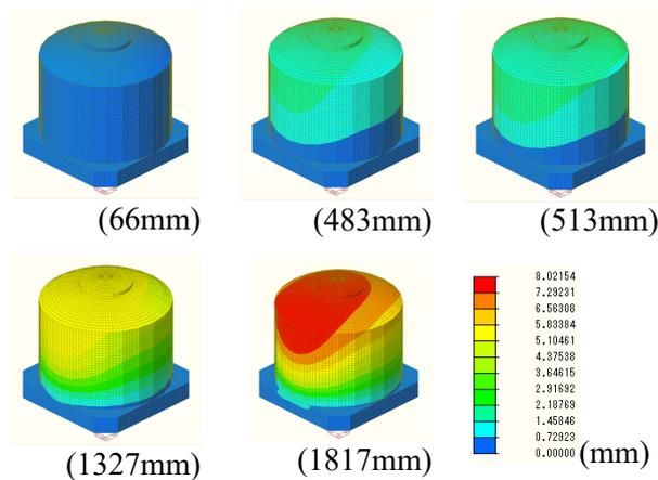
Figure 14: Tsunami wave pressure\_displacement contours
