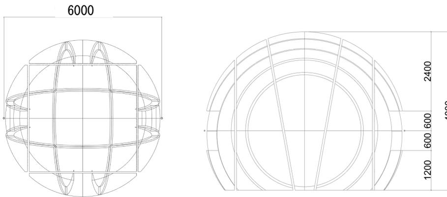
Figure 11: Floor plan of a spherical shelter
