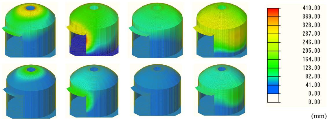
Figure 4: SAM\_Analysis Results (From left to right: roof, front, side, back / Polyurea with top, without bottom)
