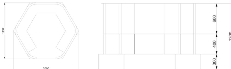
Figure 8: SAMFloat6 shelter plan
