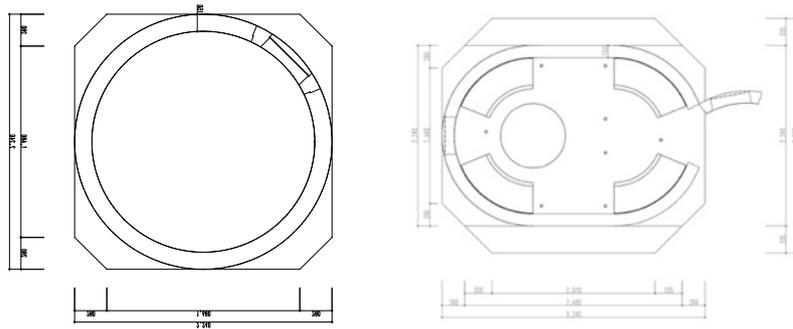
Figure 2: Tsunami shelters plan (left: SAM, right: SAMLIFE)
