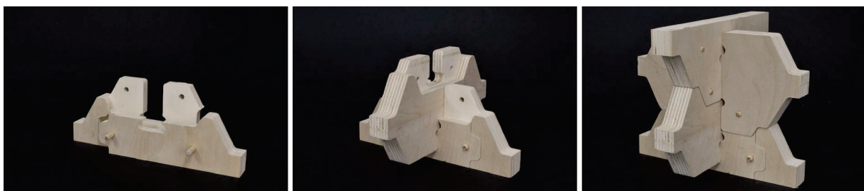
Figure 5: Joint interlocking sequence. Splice joint (left), orthogonal pieces (middle) and full joint (right).
