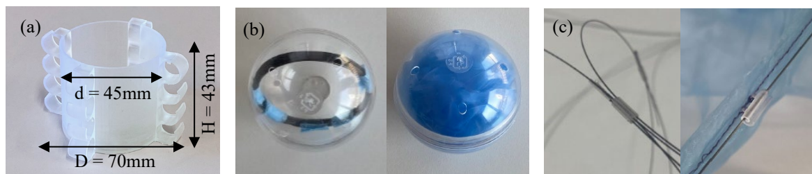
Figure 1: A – Cylindric container, B - material packed in a 7cm diameter gacha capsule, C - 3D printed parts.
