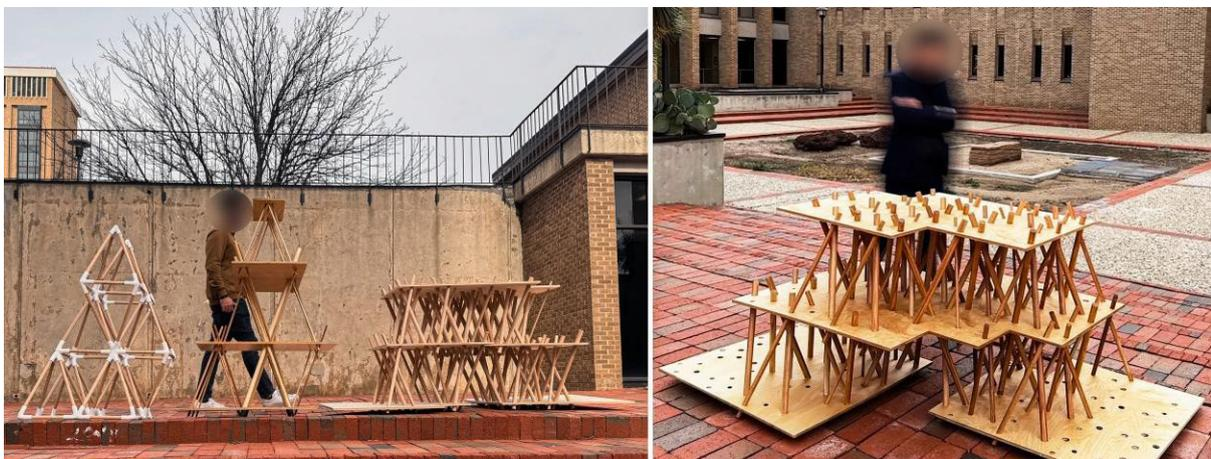
*Figure 6. Photos of one-to-one prototypes next to a human for scale. Left: the prototype features the same lattice structure but utilizes the TDRL system instead of 3D-printed joints. Right: a photograph of the manufactured and assembled prototype using oak wood for oblique dowel elements and plywood for horizontal timber elements.*
