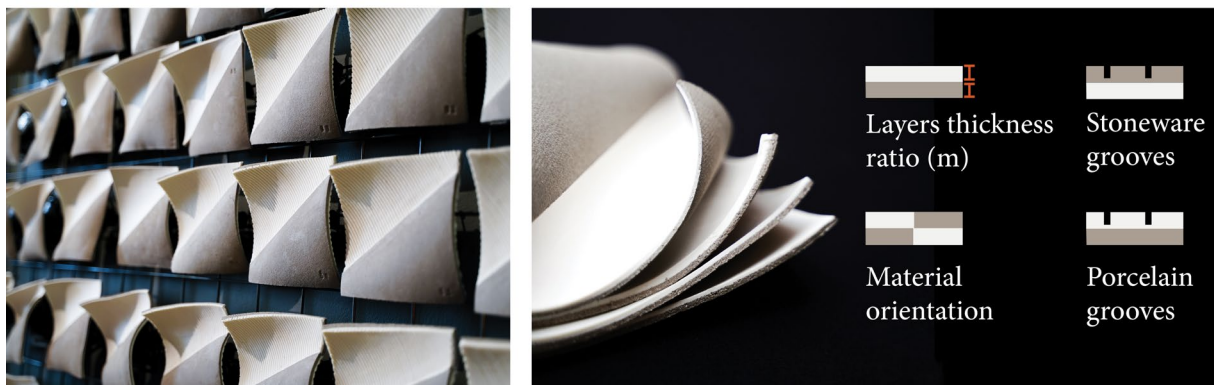
Figure 1: Complex-shaped parametric tiles exhibited in 'Creative Differences' pavilion by 'Automorph Network', at the London Design Biennale (Ofri Dar, Hagar Ofek, and Dr. Arielle Blonder), demonstrating complex control features of the FCC system as defined in this paper.
