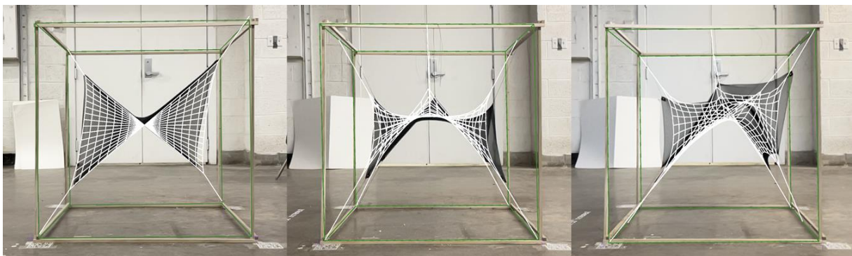
Figure 6: Form finding tensioned membranes (black textile) guided by mixed reality overlay (white and green).
