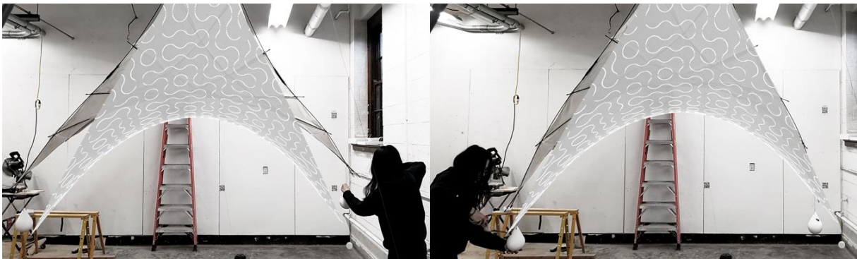
Figure 9: Adding weight to the corners of a suspended elastic frame to match target form in mixed reality. The holographic pattern aids in the visual calibration.
