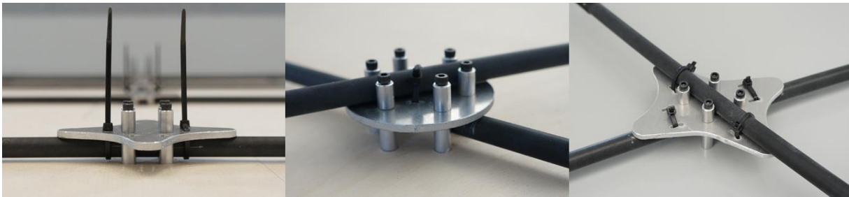
Figure 10: Plate-and-tie connections enforce intersection angle between woven rods. The longer threaded spacers attached to the bottom of the plate are set into holes in the jig, maintaining plate position during assembly.
