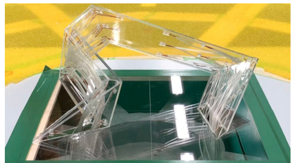
Figure 15: Test model with sensors
