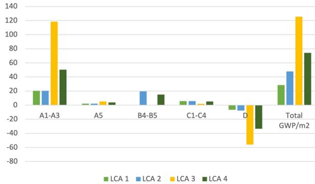
Figure 7: Comparison of LCA results per module in GWP/m<sup>2</sup>
