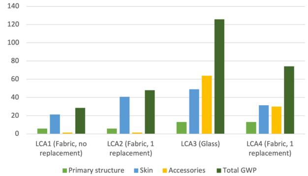
Figure 8: Comparison of LCA results per building component in GWP/m<sup>2</sup>
