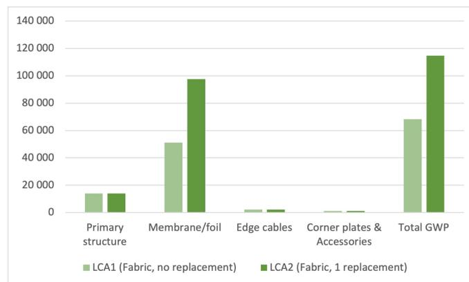
Figure 4: CS1-LCA1 & LCA2: GWP results per building element
