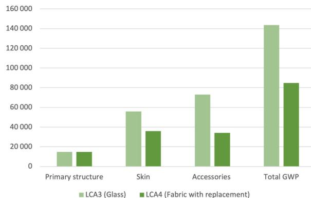
Figure 6: CS2-LCA3 & LCA4: GWP results per building element
