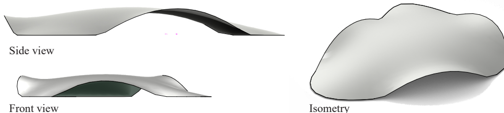
Figure 5: Geometry of shell geometry determined by form finding
