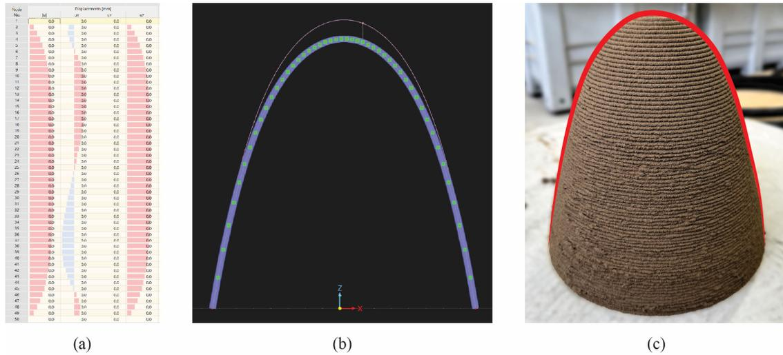
Figure 3: Deformation Analysis: (a) Displacements chart, (b) Analysis visualization (c) Printed catenary dome
