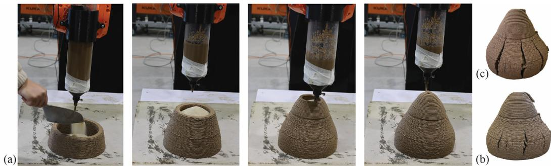
Figure 6: Second experiment of 3D printing the catenary dome with sand used for support: (a) printing process, (b) perpendicular cracks developed a short time after printing, and (c) perpendicular cracks developed after one week
