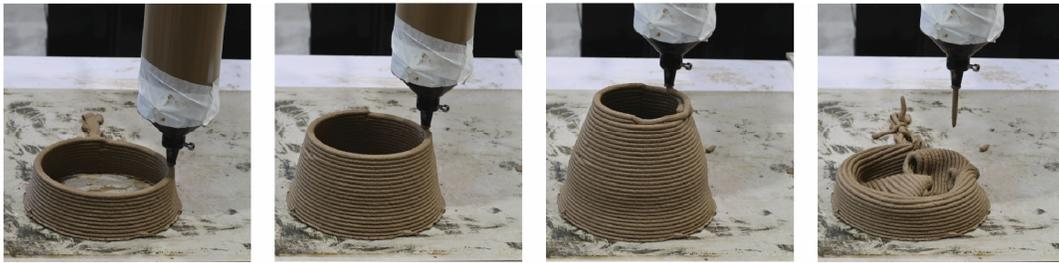
Figure 5: First experiment of 3D printing the catenary dome with stimulated soil
