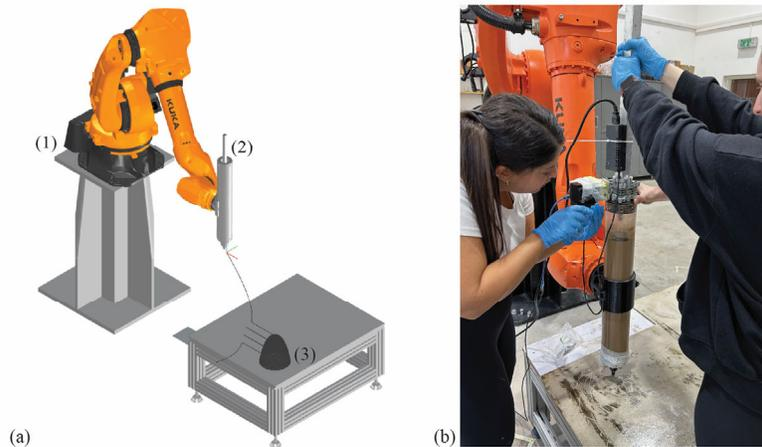
Figure 4: The experimental set up: (a) Illustration of the robotic cell comprising of the (1) Kuka KR50 robotic arm, (2) 3D Potter extruder, and (3) printing toolpath; (b) The set up preparation
