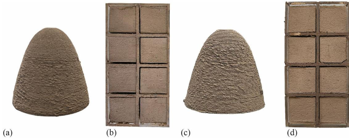
Figure 7: The 3D printed catenary domes: (a) a catenary dome 3D printed with stimulated soil, (b) 8 cast 50mm<sup>3</sup> stimulated soil cubes, (c) a catenary dome 3D printed with non-stimulated soil, and (d) 8 cast 50mm<sup>3</sup> non-stimulated soil cubes.
