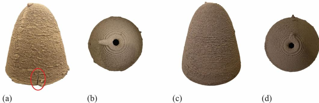
Figure 8: The 3D printed catenary domes: (a) the non-stimulated mixture dome with a crack at its base, (b) a top view of the non-stimulated mixture dome, (c) the stimulated mixture dome with no cracks, and (d) a top view of the stimulated mixture dome
