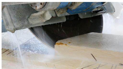
Figure 19: 5 axis cutting machine of edge angles
