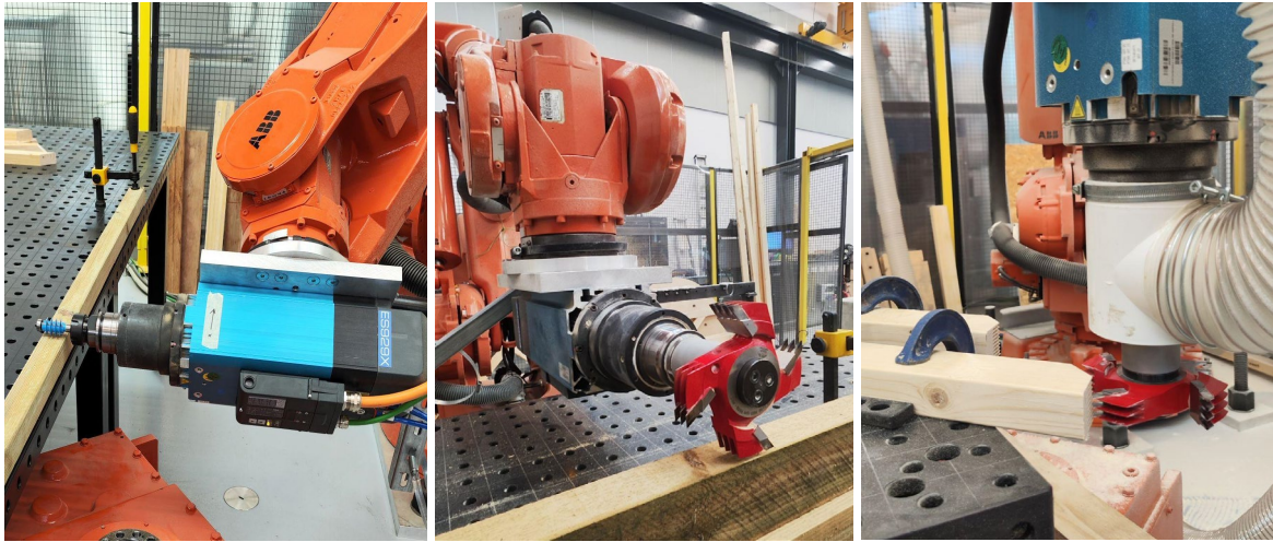
Figure 2: Robotic setup for finger joint production. Left and centre: spindle orientation for chord manufacturing. Right: spindle orientation for web manufacturing.
