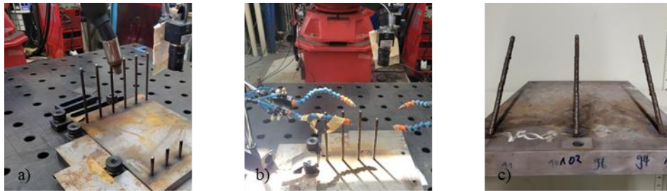
Figure 4: Manufacturing struts a) parallelly using natural cooling; b) individually using AC; c) manuf. cantilevered struts
