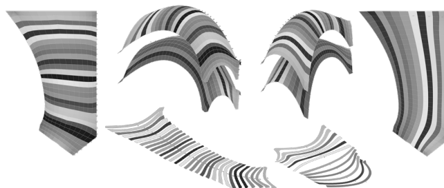
Figure 13: Constructing 3d vaulted structures from 2d warp-weft patterns
