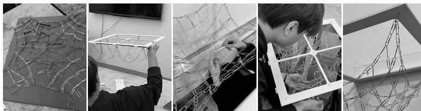
Figure 6: Using paper clips for rapid assembly of low-fidelity catenary vaults under tension
