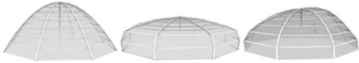
Figure 2: The investigated configurations: the paraboloid (left), the ellipsoid (middle) and the teardrop (right)
