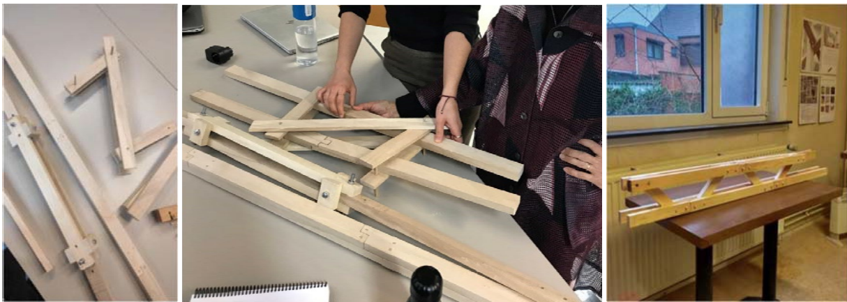
Figure 7. Phase 2 prototypes: 1:2 models exploring lamination with wooden dowels to create truss elements.
