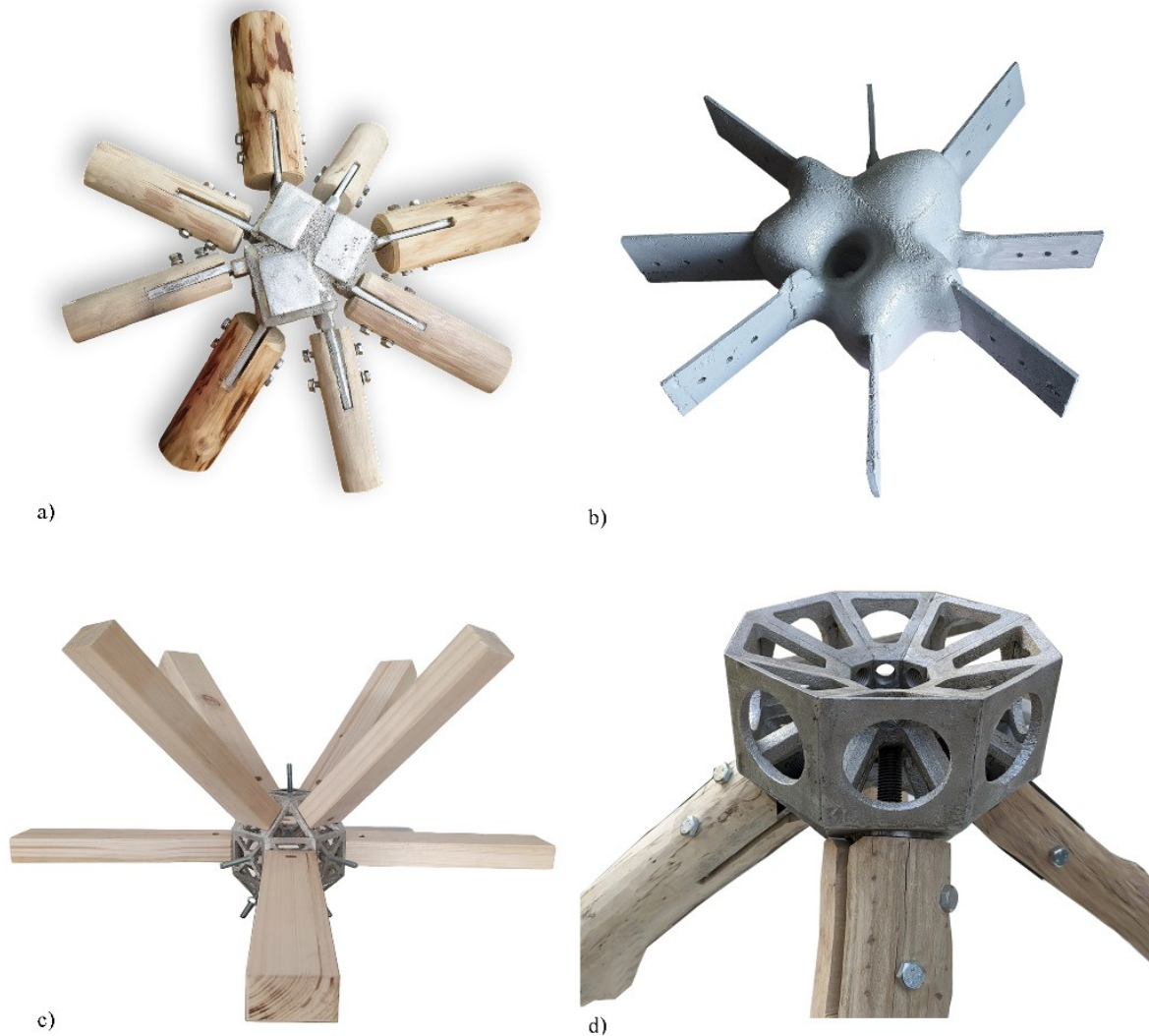
Fig. 3: A number of prototypes were developed, ranging from topology optimized nodes (a, b) to the final modular approach (c, d).
