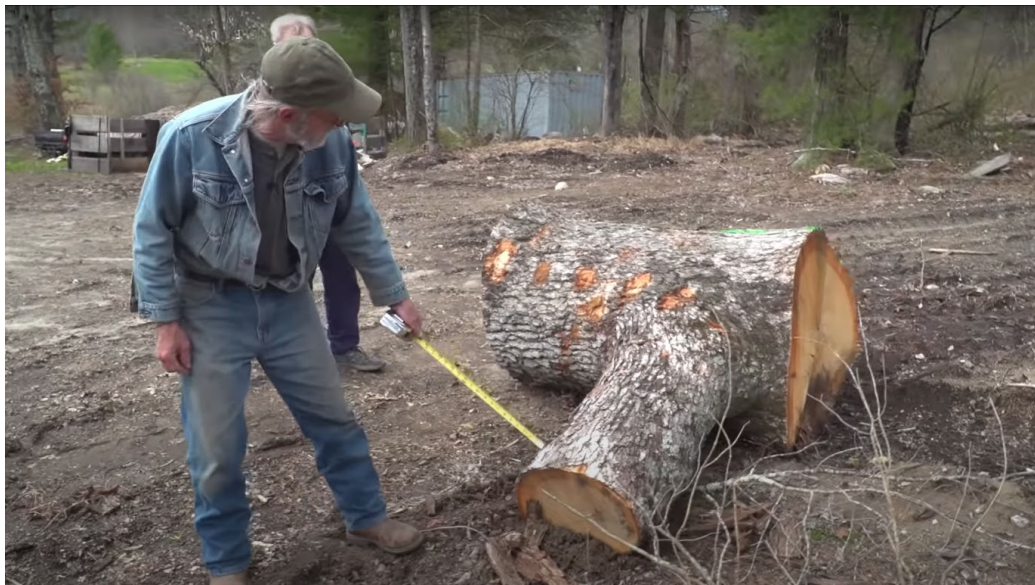
Image 1: Louis Sauzedde analyzes a tree fork that he will use for brace knees [Sauzedde 2020]
