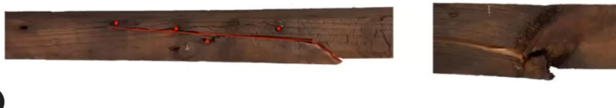
Image 2: Chris Humphrey's use of Canny Edge Detection to predict structural failures in recycled boards [Humphrey 2023]
