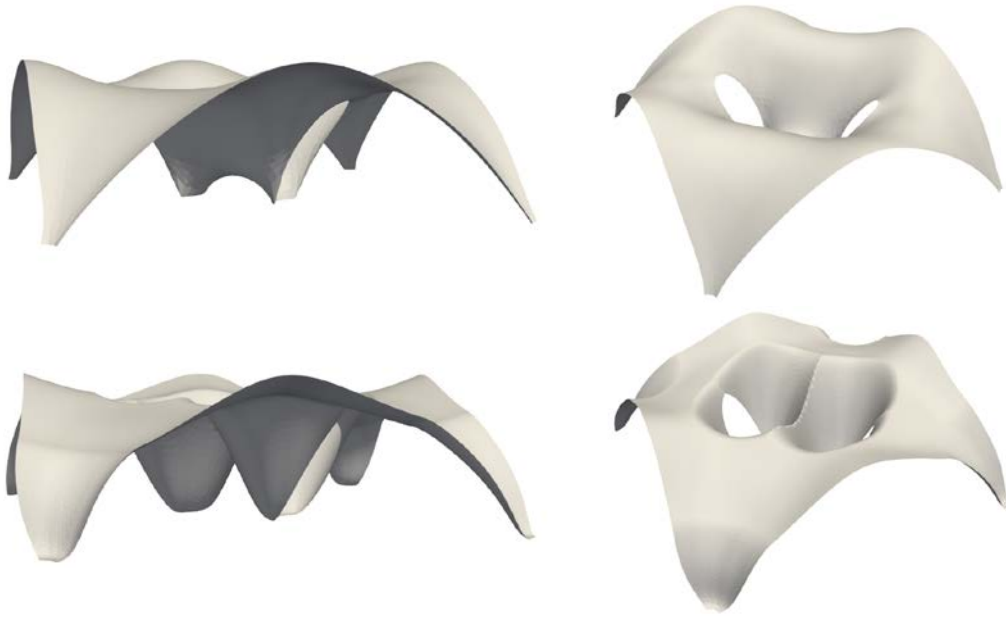
Figure. 11, continued: Free form shell on quadratic plan. Top: results with implicit filter and large radius; Bottom: result with explicit filtering and small radius.
