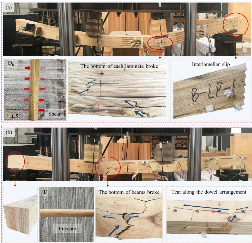
Figure 7: Failure modes of DLVL beams: (a) B-LP; (2) B-LV
