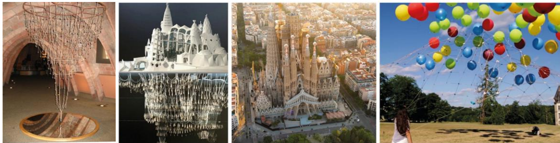
Figure 6: The funicular explained to children, with the examples of a suspended chain model from Casa Milà [Alexandre Borovik], a scale model of the crypt from Park Güell compared to the Sagrada Família of Antoni Gaudí (1852-1926), and the floating dome by P. Block at Bois Buchet [Zito Tseng CIRECA].
