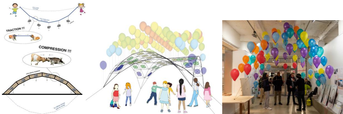
Figure 7: The funicular and its sensitivity to the position of loads [Les Petits Constructeurs 2].
