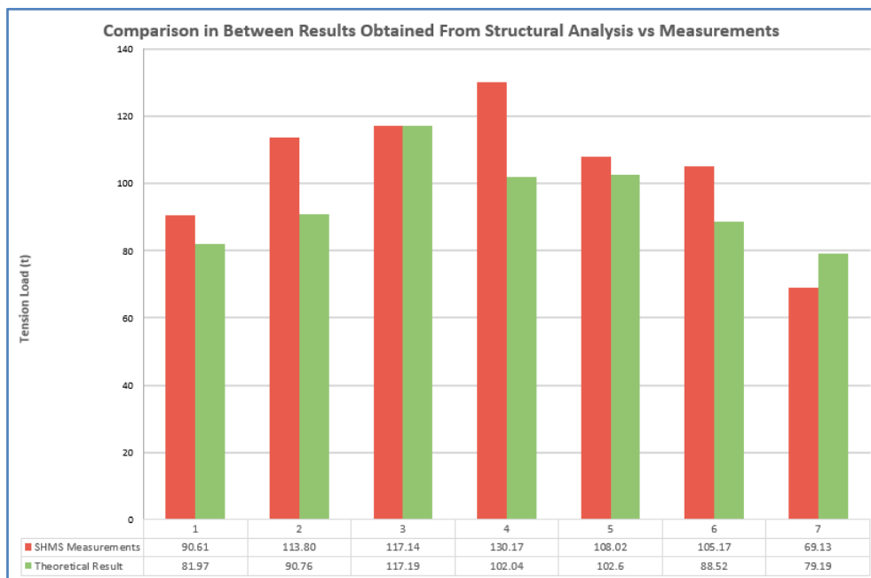
Figure 10: Comparison in between results obtained from SHMS and theoretical results (with roof cladding)
