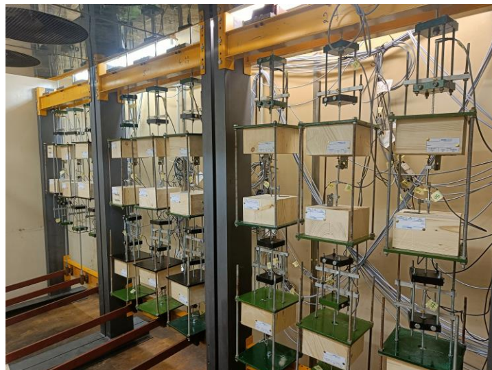
Figure 7: Experimental setup preparation for the constant climate long-term tests in climatic chamber
