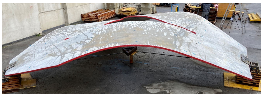
Figure 8: Crack pattern on the surface
