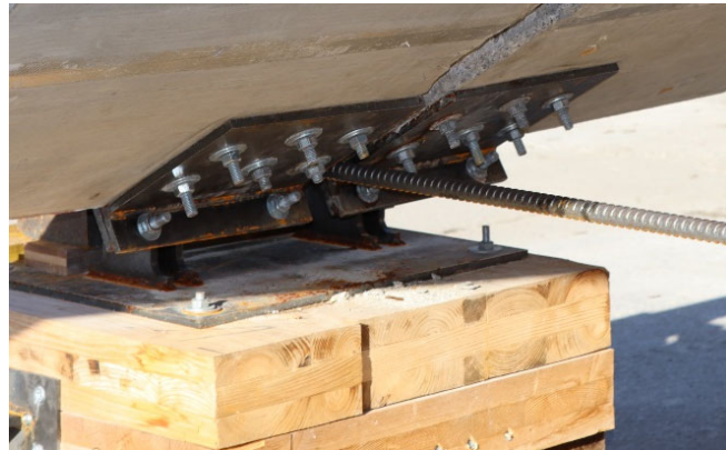
Figure 4: Hinged roller support
