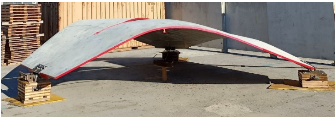
Figure 6: Actively bent concrete shell – side view
