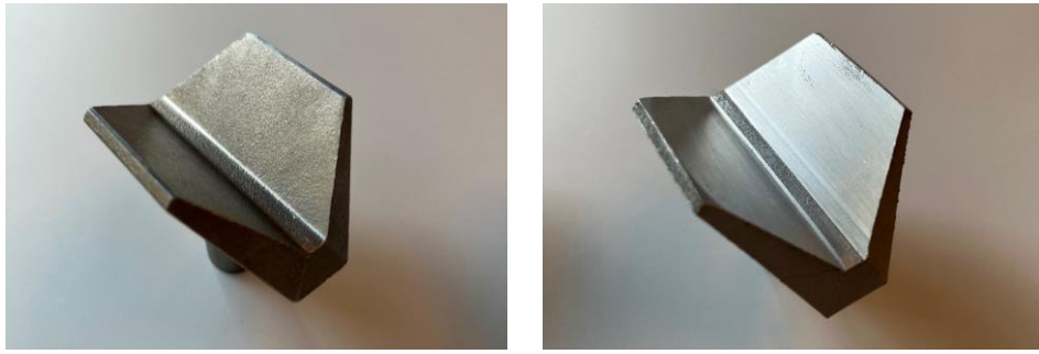
Figure 6: Brut wax-casted connector and rectified connector
